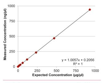
Figure 2: Samples (mean value) in the range of  $1.89 - 932 \text{ ng/}\mu\text{l}$  were measured with path length 0.67 mm.
