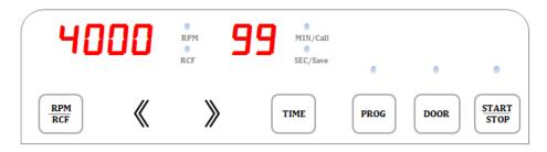
[RPM/RCF]: Use to set the rotor speed and for RPM/RCF conversion
